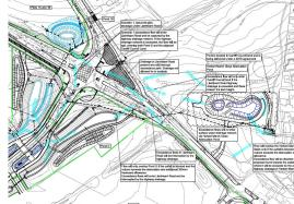
Click <u>here</u> to open the image full size The double ponds are on the right hand side of this diagram near the gardens of Herbert March Close. The temporary vehicle only access situated within the precinct of a Toucan crossing on Llantrisant Road will be made permanent for Council Parks maintenance or emergency access.
